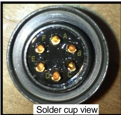
[left] Solder cup pins on back of standard control plug. Pin orientation matches the schematic above, and is marked on the inner face of the plug itself. When assembling the Std. connector, remember to pre-position wires thru the strain clamp, plug shell, and shrink wrap before soldering.
