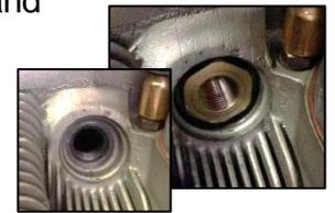
**Note:** [Continental] LRX is an LR adapter with the hex head extended 1/4" to facilitate socket attachment (removal only) on Continental 550s (maybe others) where the plug hole is recessed – see pic.
