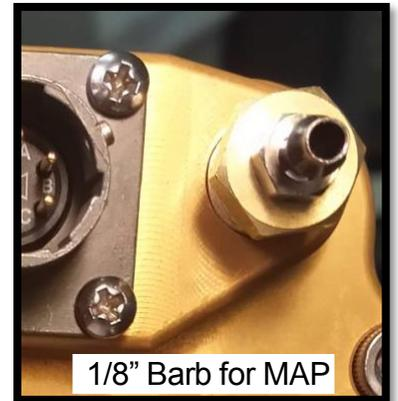
With **normally aspirated** engines, the MAP tube is a fail-safe input. Meaning if the MAP plumbing comes loose or fails, plug firing in NORM Mode will retard to a very flyable, but slightly less efficient, firing position. If installing two ignitions, run a single MAP tube to the accessory area, and then tee the line to each ignition. If you have a manifold pressure gauge, tee into that existing line for your pressure source.
