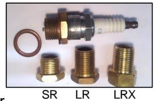
Note: [Continental™] LRX adapter is an LR adapter with the hex head extended 1/4" to facilitate socket attachment (removal only) on Continental™ 550s, and possibly others, where the plug hole is recessed, and standard sockets may not reach.
