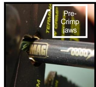
In either case, **if you don't feel and/or hear the terminal snap**, remove and inspect for irregularities or damage. If needed, replacement terminals can be provided by E-MAG.
