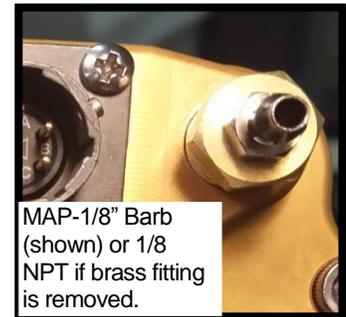
With **normally aspirated** engines, the MAP tube is a fail-safe input. Meaning if the MAP plumbing comes loose or fails, plug firing in Variable Mode will automatically retard to a very flyable, but slightly less efficient, firing position. If installing two ignitions, run a single MAP tube to the accessory area, and then tee the line to each ignition. If you have a manifold pressure gauge, tee into that existing line for your pressure source.
