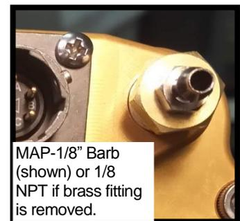
With **turbo normalized or boosted** engines, **MAP plumbing is NOT considered fail-safe**. A MAP plumbing failure can, in certain conditions, call for more ignition advance than is appropriate or safe. Excess advance can result in loss of power, overheating, and/or damage to the engine. For this reason:
