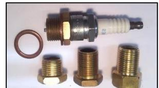
*LRX adapters have extended hex heads to facilitate removal from some certain engines (550s and maybe others) where the plug seat area is recessed and too tight for standard sockets. **When needed, you must specify LRX adapters when ordering.***
